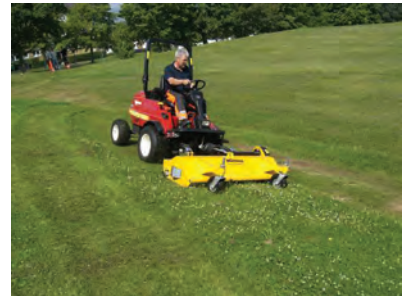
Fig 61. Flail mower consists of small, hinged T-shaped flail blades mounted on a spinning shaft (flail shaft).
